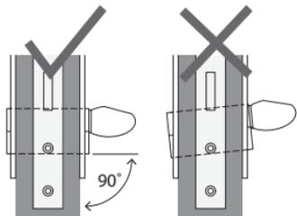
3. **DO NOT FORCE** the cylinder into place as this will damage the cylinder and lockcase and invalidate the warranty.
