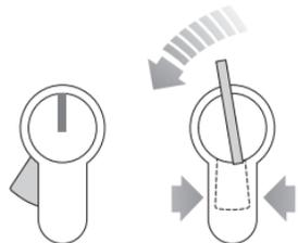
2. Insert the cylinder into the lock case making sure it is horizontal and at 90° to the door face before fully tightening the escutcheon/backplate fixings.
