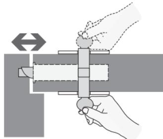
6. Ensure the door latches correctly and that the deadbolt (if appropriate) throws smoothly into the keeper. Adjust strike plates accordingly.
