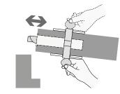
G. Ensure the door latches correctly and that the deadbolt (if appropriate) SCrew. throws smoothly into the keeper.
